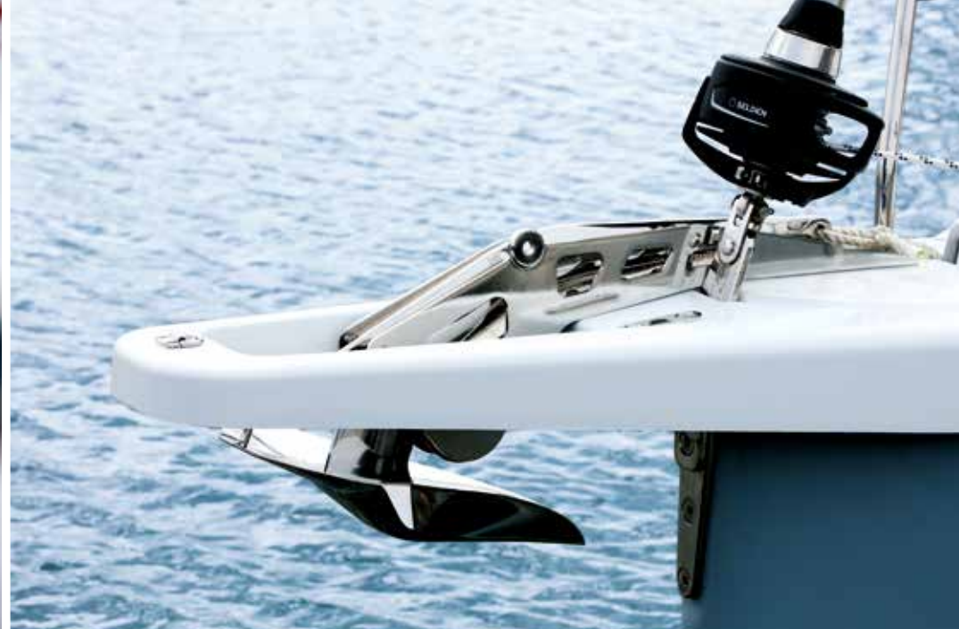
The optional bow sprit increases the sailing performance with asymmetrical headsails.
