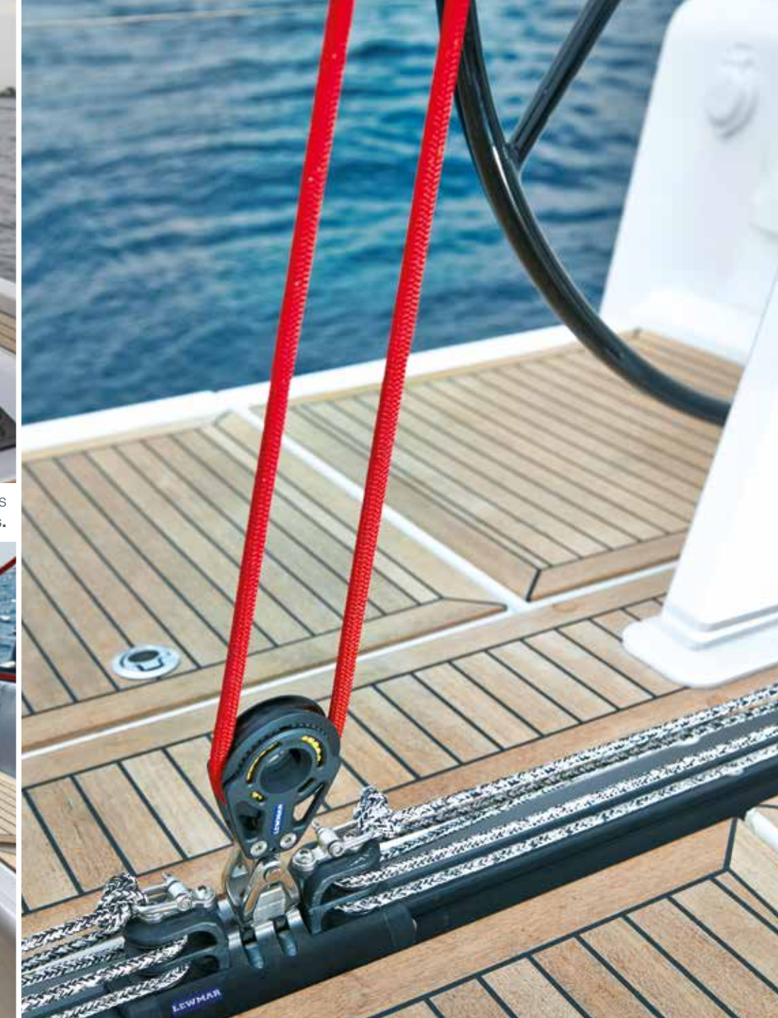
Recessed into the floor, the mainsheet traveller allows an ideal trim of the mainsail.
