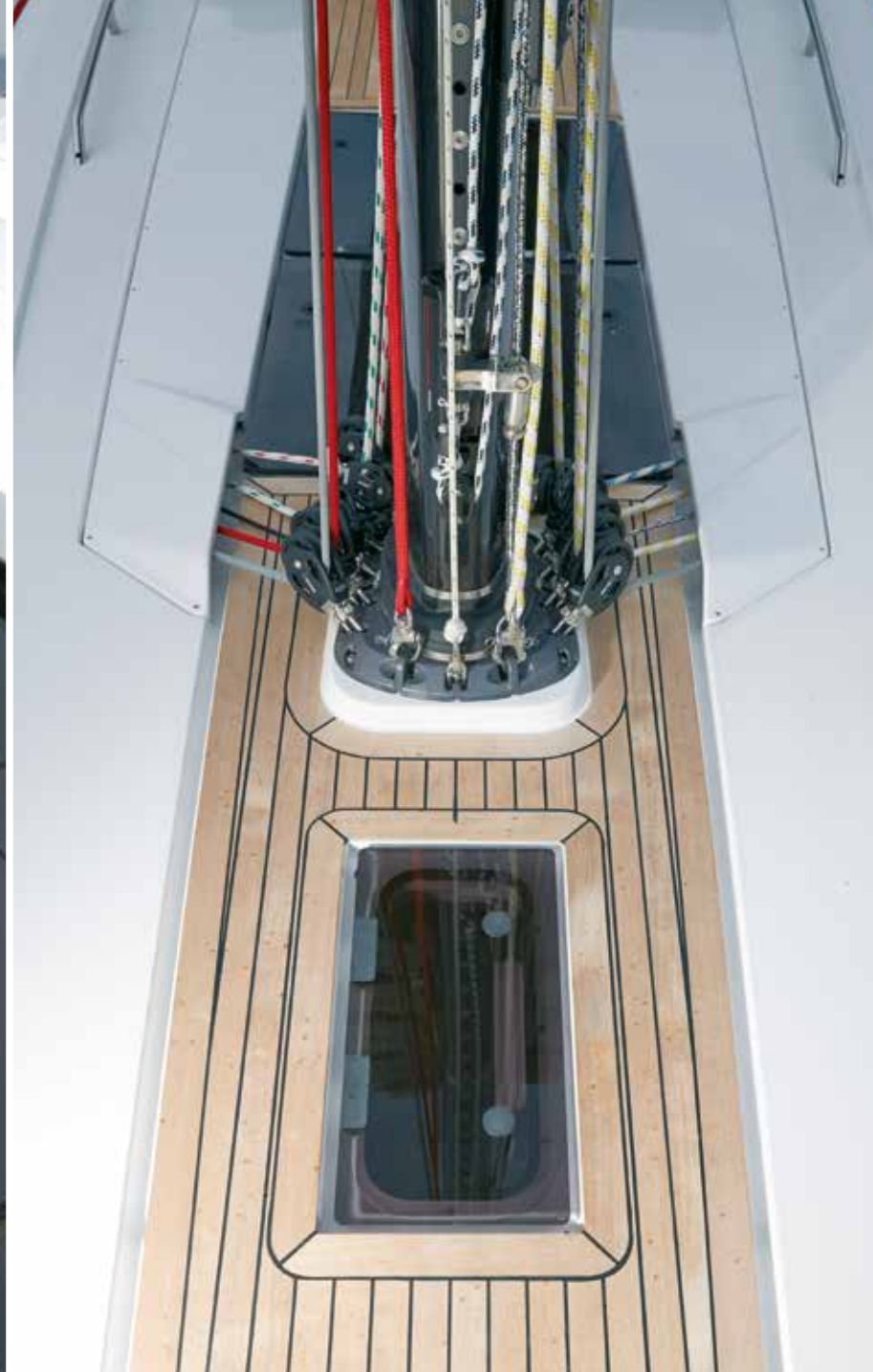
Hidden halyards allows the deck design to be clean-cut.
